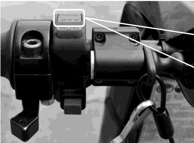
**Battery disconnect:** *stops battery discharge.*
