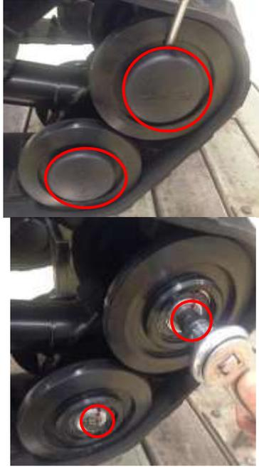
2. Take off the large bogey wheels and take the track off. Use an Allen key to loosen the 4 x M5 bolts which fasten with the right suspension.
