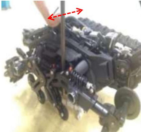
10. Right side suspension removal is completed. Next, install a new chain.
