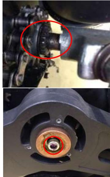
15. Install steering linkage, but don't tighten the nuts for adjusting the steering.
