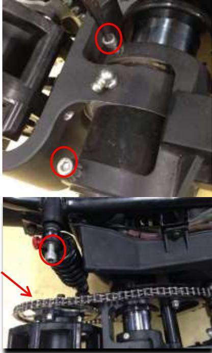
14. Adjust the position of the engine and gearbox to combine steering arm and steering shaft smooth, and tighten the bolt.
