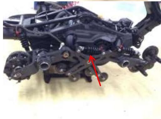
13. Tighten the right suspension with four bolts into the pivot tubes. Install the chain. Apply industrial grade Red Loctite on the rear shock bolt before assembling it.
