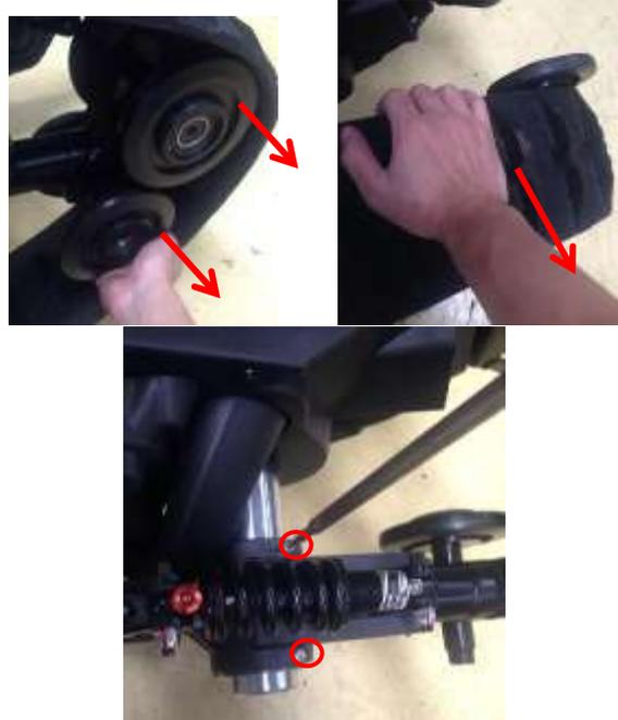
3. Use a 12mm wrench to loosen the chain tensioner nuts, and use a 14mm and 17mm wrench, loosen the drive sprocket bolts.
