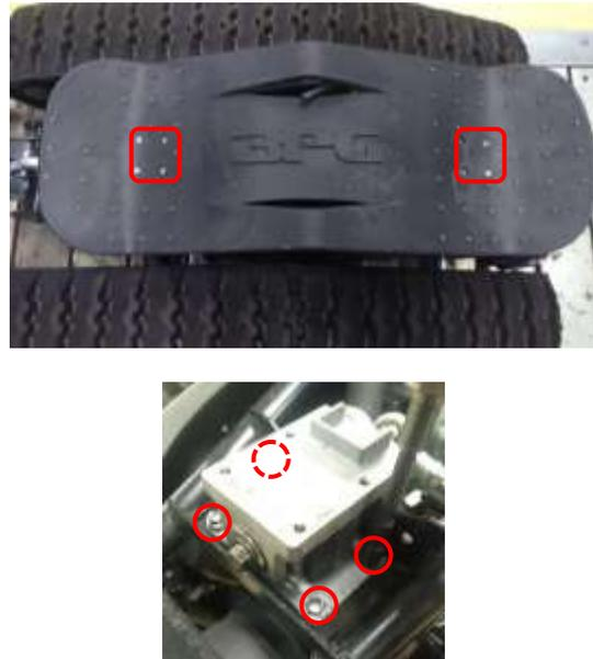
5. Use a 10mm wrench to loosen the steering link nuts, and take off the steering rod.
