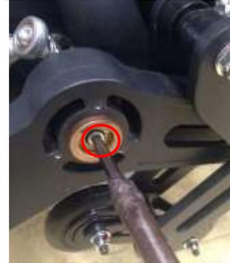
7. Use 10mm wrench to loosen upper bogey wheel arm and use 6mm Allen key to take off the rear shock bolt.
