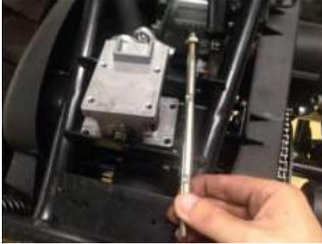
6. Use a 3mm Allen key to unscrew 3 dust cap screws and take off the dust cap. Then use 8mm Allen key to loosen the socket head bolt of steering rod.
