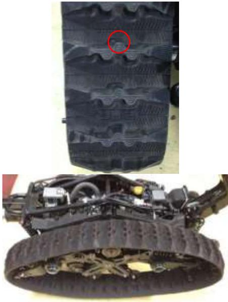
18. Rotate the track to help slide it onto the inside big bogey wheel, and then mount the outside big bogey wheels. Insert and tighten the bolts back on with their respective washers and plates and put the bogey wheel covers back on. Follow the chain and tracks adjustment guides to make sure your DTV is at optimal setup.
