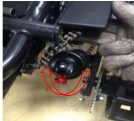
9. Pull out the right suspension assembly by hand or use a bar for leverage to help the assembly slide off.
